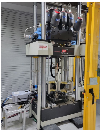
Figure 4, High Strain Rate Tensile Experiment setup
