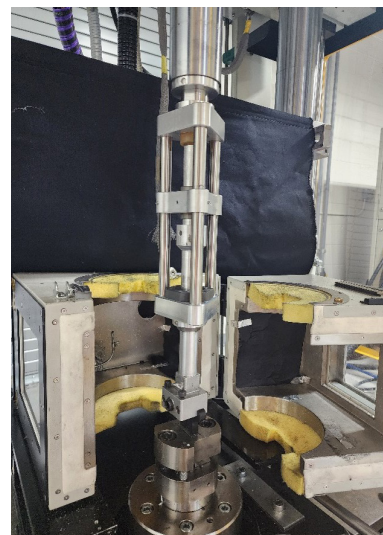
Figure 5, High Strain Rate Slack Grip apparatus
