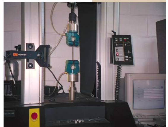
Figure 10: Simple Tension Test with Video Extensometer
