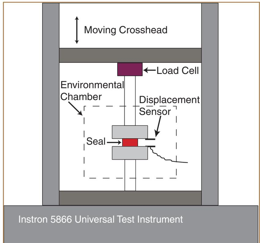
Figure 7, Schematic of Experimental Apparatus used to Measure Seal Pressure During Thermal Changes
