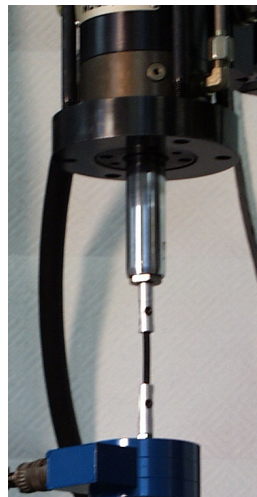
Figure 8, Tension Specimen in Servohydraulic Test Instrument
