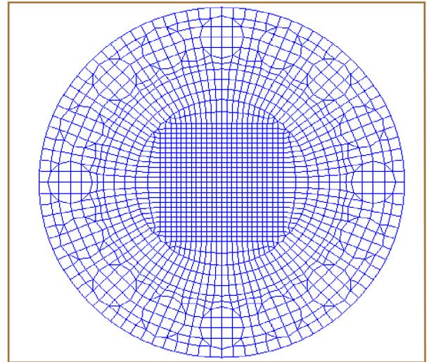
Figure 4, FEA model of uncut specimen with radial loads applied at every perimeter node.
