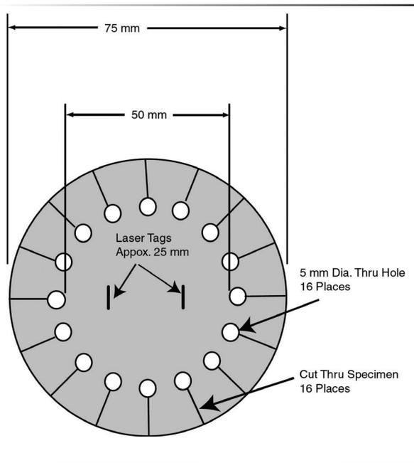
Figure 3, Biaxial Test Specimen Outline
