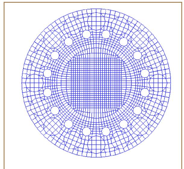
Figure 5, FEA model of specimen with slits and punched holes, radial loads applied at 16 grip locations.
