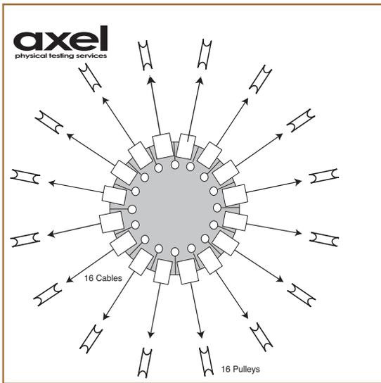
Figure 2, Biaxial Apparatus Schematic
